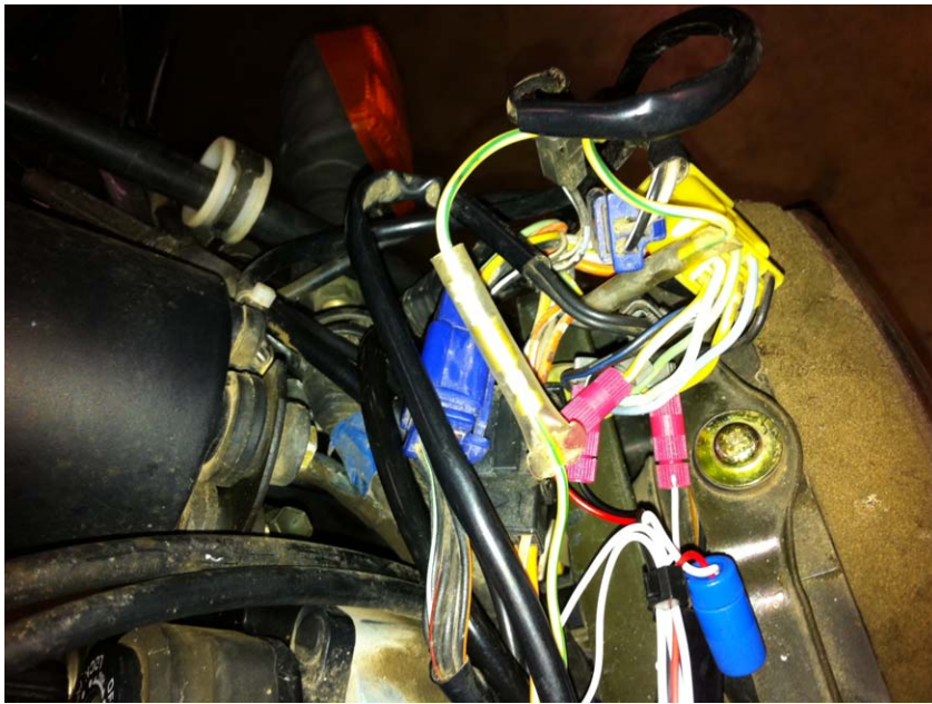
Relay box mounting location suggestion.
