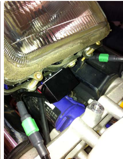
Relay box mounting location suggestion.
