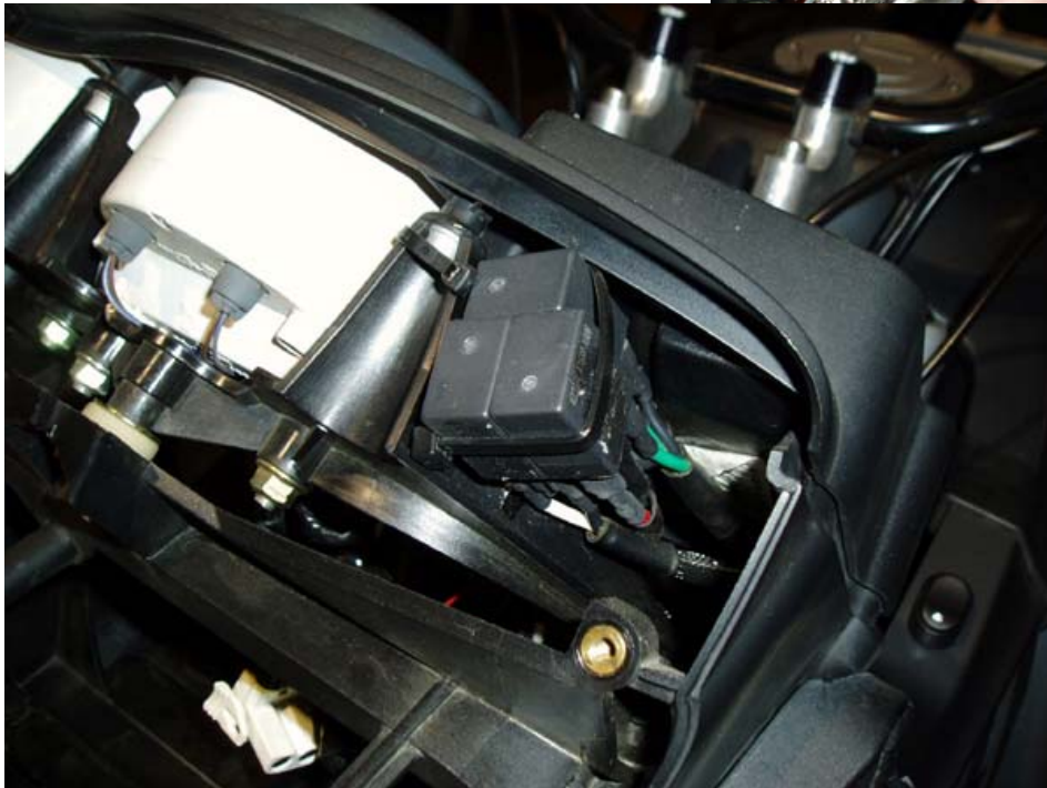
Relay cluster location. Note: new version of harness has 2 relays instead of 3.
