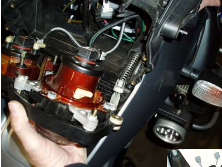
Headlight adjuster connection. Note: Ballast and bracket not shown.
